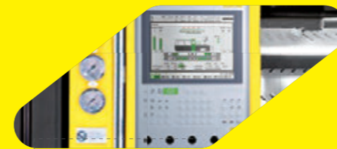
Automatic control Austria made KEBA controller model 2880
