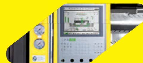
Automatic control Austria made KEBA controller model 2885
